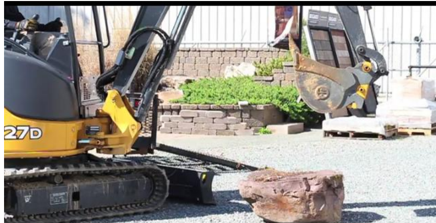
Align the bucket or forks with the boulder
